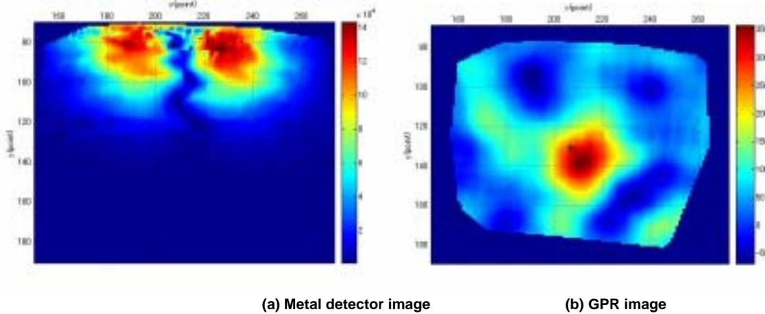
Fig.2 Typical ALIS output image of buried AP landmine. (PMN-2, 10cm depth)
