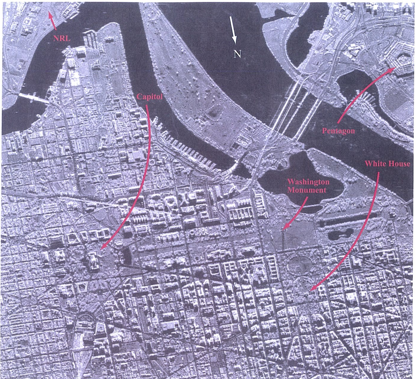
Figure 1-19: This figure presents a Ku-band SAR image collected over Washington, D.C. The SAR illumination is from the top. Man-made features, such as buildings and bridges, stand out clearly in this radar backscatter image. The backscatter intensity of water is much smaller than that of buildings and vegetation, so water shows up black in the image. Individual trees can be distinguished in some areas, and the pattern of roads and urban development is clearly apparent. The Capitol building is left of center with the Mall extending to the right. Right of center is the Washington Monument, though only the shadow of the obelisk is readily apparent in the image. Just below the monument are the Ellipse and the White House. The Naval Research Laboratory is at the upper left. [Courtesy of Sandia National Laboratory.]
