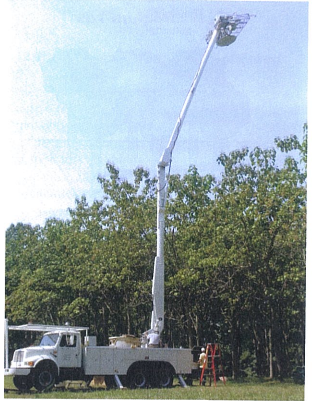
Figure 11-48: 1.25 GHz radar system deployed over a stand of Paulownia trees [Kurum et al., 2009].
