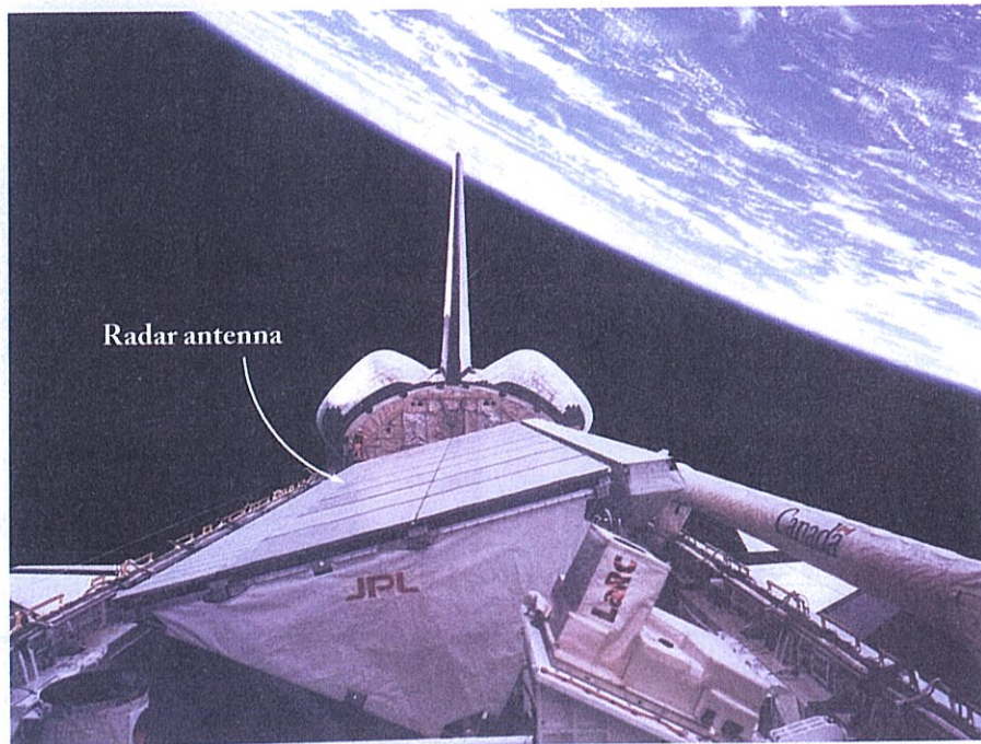
12 m long SIR-C radar antenna carried by the Space Shuttle
