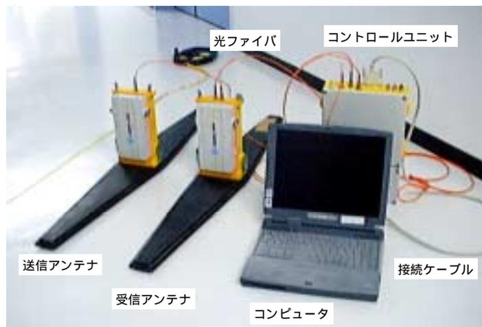
Fig.3.6 GPR system with separated components (RAMAC GPR with the 100MHz Antenna)
