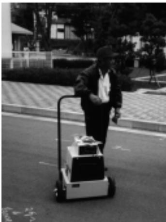
Fig.3.5 GPR system with unified components (KODEN GPR)
