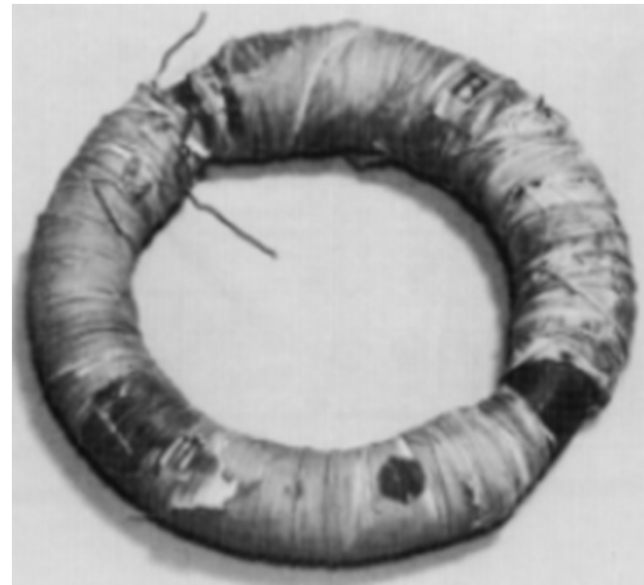
The first transformer: Two coils wound on an iron toroid.
